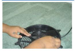
Ensure Fan Assy. is properly seated onto shaft alignment pin.
