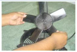
Pull Fan Blade Assy. up off of shaft, rotate 180° then place back onto shaft.
