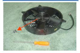
Carefully remove Fan Assy. Retaining Clip.
