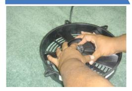
Snap Retaining Clip back into its original position.
