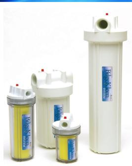
The patented BilgeKleen System automatically removes oil, gas, diesel fuel and other hydrocarbon pollutants from bilge water before it is discharged overboard. Using a special filter medium, the BilgeKleen captures and binds to hydrocarbons and lets water pass through freely. As a result, 99.9% of the hydrocarbon pollutants are eliminated from discharge with no increase in pressure to the bilge pump.
